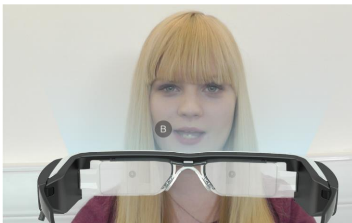
Figure 10: A rendering of the current iteration of PhonemeViz, showing what would be displayed on the Epson Moverio Glasses for the word "Bat".
