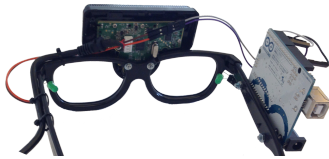
Figure 2: Prototype with microphone array at centre of a pair of eyeglasses and peripheral LEDs connected to an Arduino.
